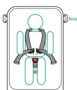
C. Ensure slack is removed from shoulder harness strap by pulling lap straps then pull the Harness Adjustment Strap to take up the slack in the harness adjusting to a firm but comfortable fit. Make sure that nothing is obstructing the harness straps and that baby's arms and legs are free. Check that slack in straps is minimal. Do not use the restraint if straps do not tighten and contact your local authorised service agent for repair.
